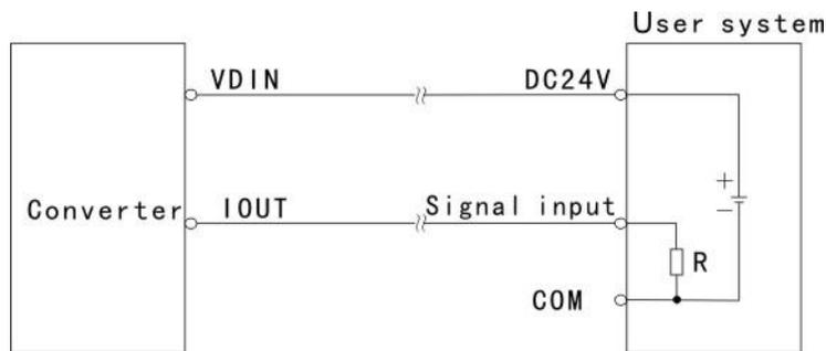
1.6a Two-wire system wiring method (Square converter)
