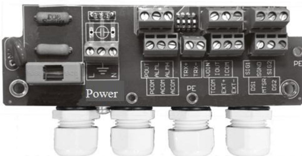
Fig. 1.3 (a) Wiring terminal diagram of square meter
