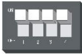
Switch1: ON supply upper power(24V) for ALML alarm output. OFF is no connection.
