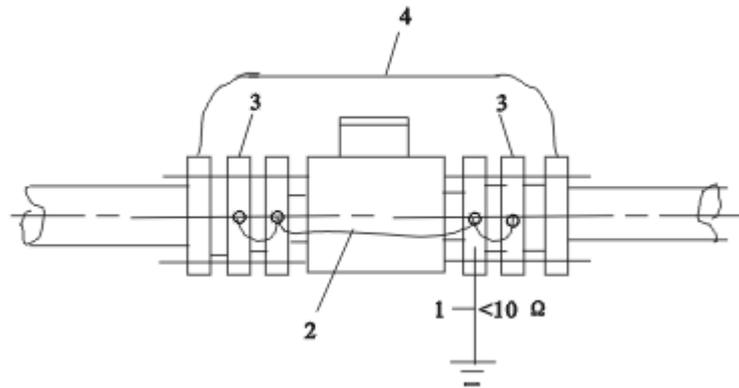
Fig.7.5.2 Installation method of the sensor is on pipeline with cathode protection potential
