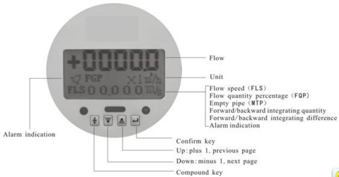
Fig. 1.2.1 Keyboard definition and liquid crystal display of circular meter
