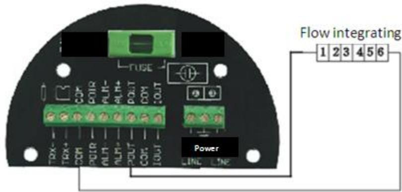
Fig. 1.4 (g) Electronic counter wiring of circular meter
