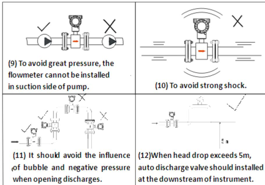
Fig. 7.2 Graphical representation electromagnetic flowmeter installation
