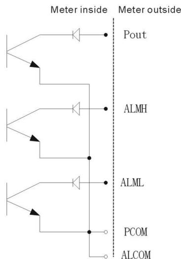
Fig. 1.4 (i) Meter inside OC gate connection mode
