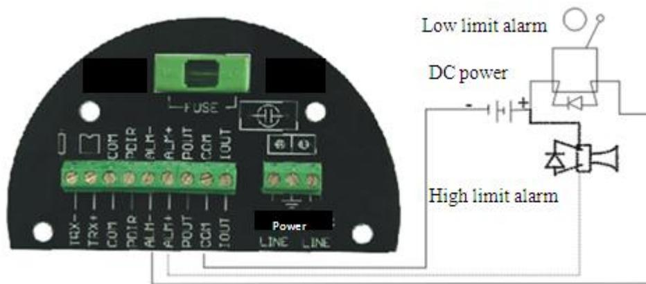
Fig. 1.4 (h) Alarm output wiring of circular meter
