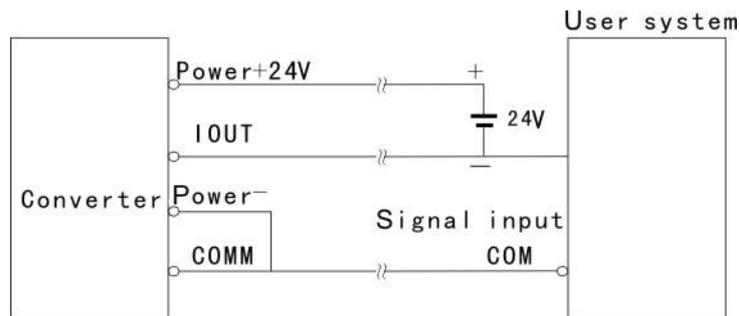
1.6b Three-wire system wiring method (supply power and current output isolation mode)
