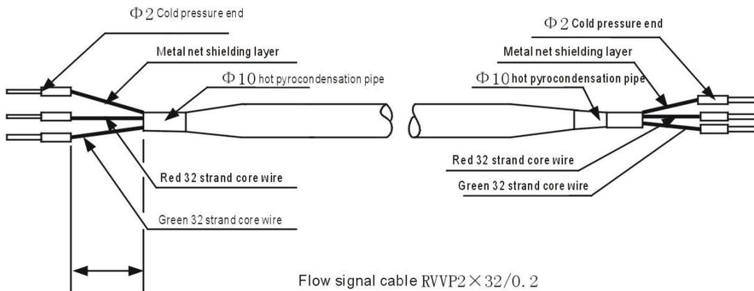
Fig. 1.3.2 Signal wires processing and labels of connection of square meter and sensor
