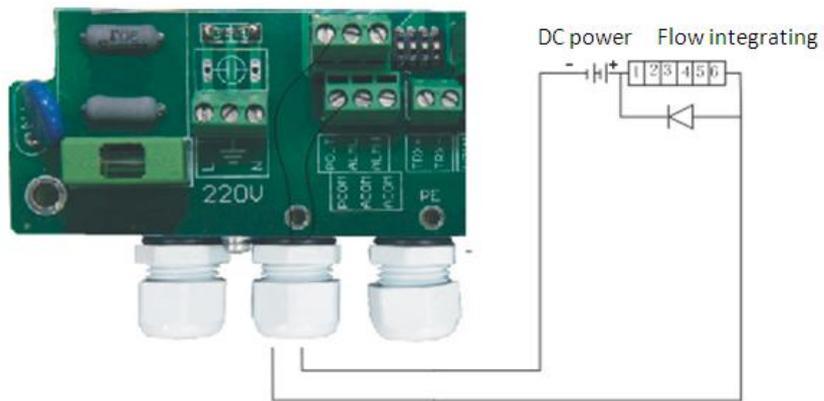
Fig. 1.4 (b) Electromagnetic counter wiring of square meter
