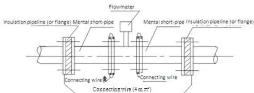
Fig.7.5.3 Installation method on the pipeline with large working frequency current
