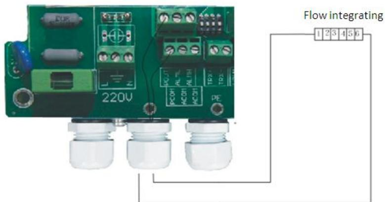
Fig. 1.4 (c) Electronic counter wiring of square meter
