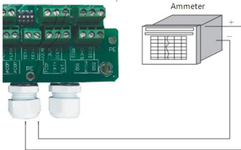
Fig. 1.4 (a) Wiring diagram of square meter current output
