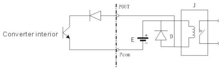
Fig. 1.5 (c) Digital quantity output connects relay
