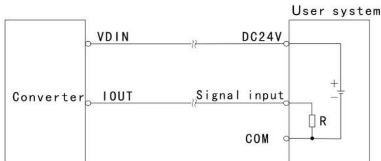
1.6a Two-wire system wiring method (Square converter)
