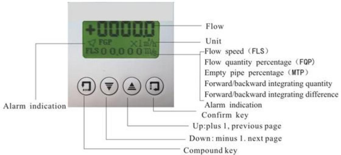
Fig. 1.2.1 Keyboard definition and liquid crystal display of square meter
