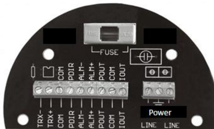
Fig. 1.3.3 Wiring terminal diagram of circular meter
