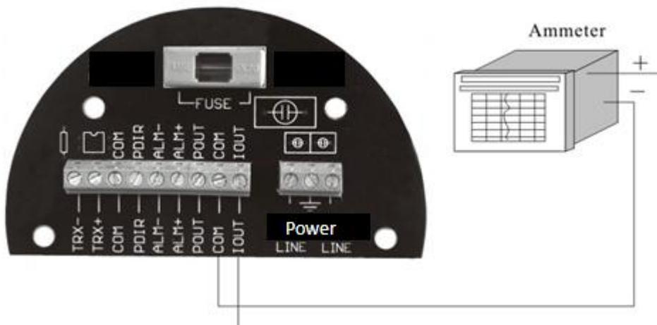
Fig. 1.4 (e) Wiring diagram of circular meter current output
