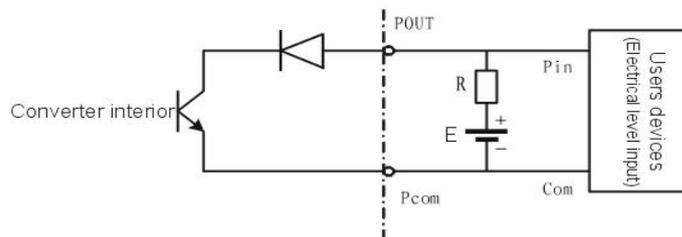
Fig. 1.5 (a) Digital quantity electrical level output wiring method
