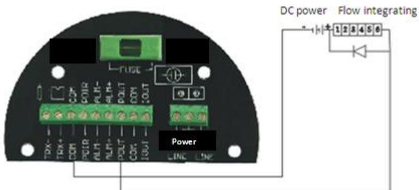
Fig. 1.4 (f) Electromagnetic counter wiring of circular meter
