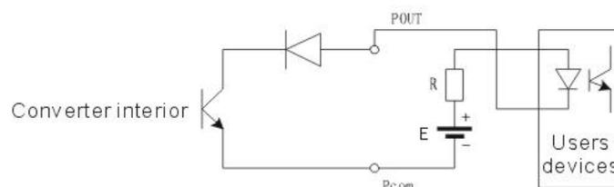
Fig. 1.5 (b) Digital quantity output connects photocoupler
