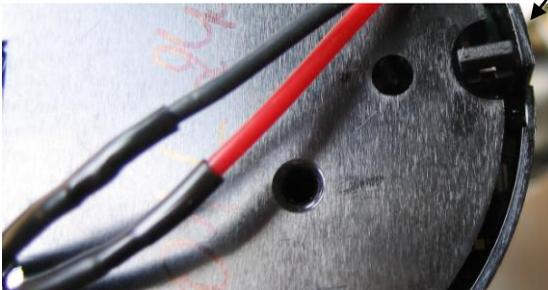
Fig. 5. Back lighting jumper view at transmitter electric board (unit display back side).
