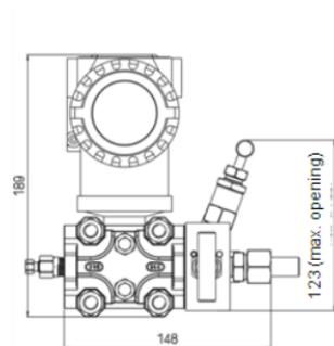
Dimension (with T3 series 3-valve manifold)
