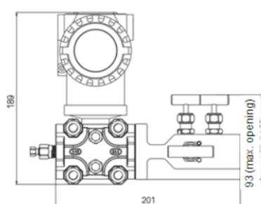
Dimension (with V5 series 5-valve manifold)
