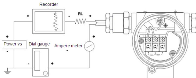
Fig. 7-1 External wiring diagram of BPT361 series intelligent transmitter
