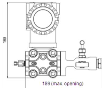
Dimension (with V2 series 2-valve manifold)
