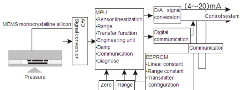
Fig. 1-1 Block diagram for working principle
