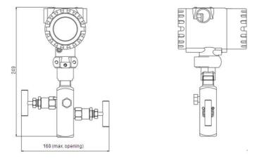
Dimension (with V2 series 2-valve manifold) (Unit: mm)
