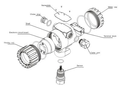
Fig. 5-1 Parts of BPT362 series pressure transmitter
