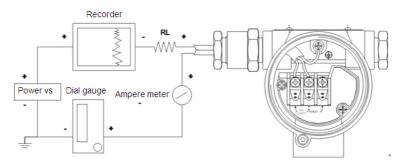
Fig. 7-1 External wiring diagram of BPT362 series intelligent transmitter
