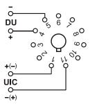
Reversed UIC-voltage polarity is shown in brackets!
