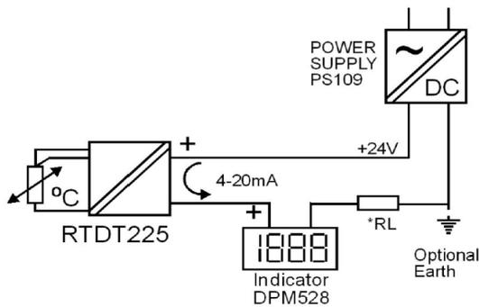
\* NOTE RL is input load of PLC, VSD, or other process instruments.
