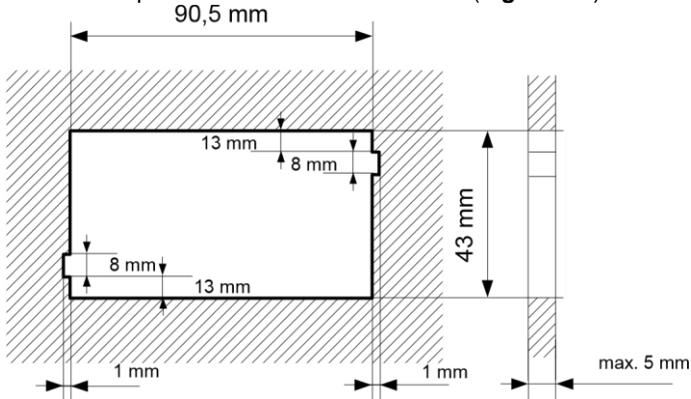
Figure 4.1. Recommended mounting hole dimensions 92
