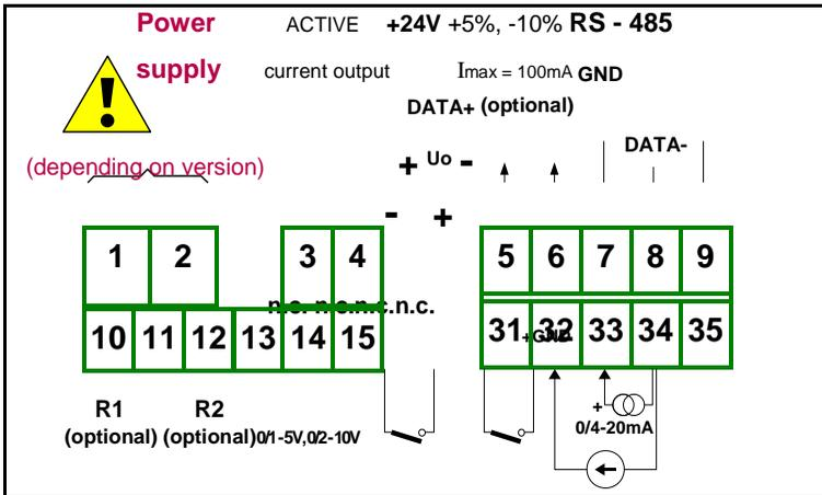
Figure 4.8. Terminals description (relay and active current outputs)
