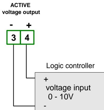
Figure 4.22. Example of active voltage outputs connection (for device with active voltage output only)
