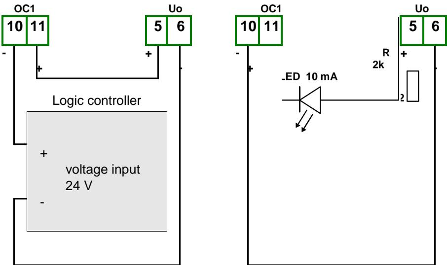
Figure 4.19. Example of OC-type outputs connection
