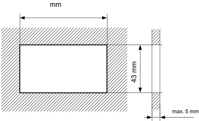
Figure 4.2. Allowable mounting hole dimensions
