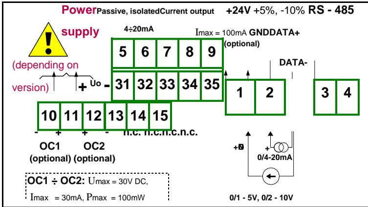
Figure 4.11. Terminals description (OC-type and passive current outputs)
