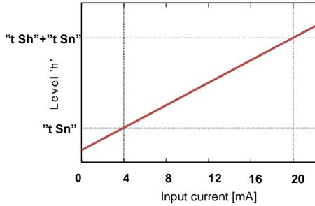
Figure 10.5 The characteristic of level of liquids, gases or solids in tank depending on input current in 4-20mA range.
