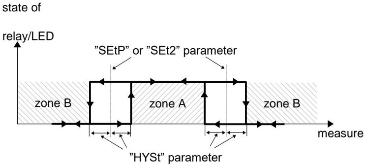
Figure 6.5. Two threshold control of the relay/LED outputs
