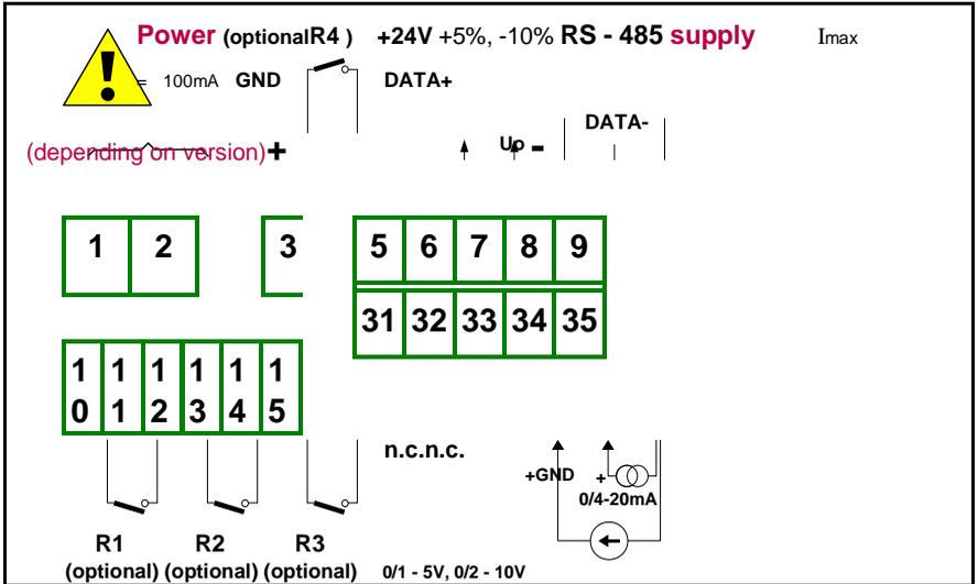
Figure 4.6. Terminals description (relay outputs)
