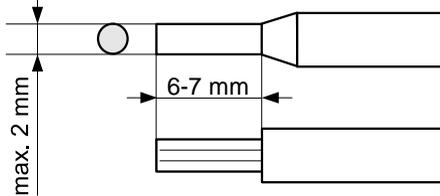
Figure 4.5. Method of cable insulation replacing and cable terminals
