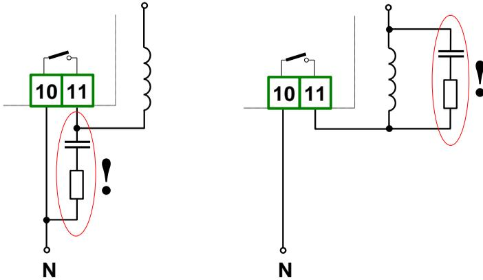
Figure 4.18. Examples of suppression circuit connection:
