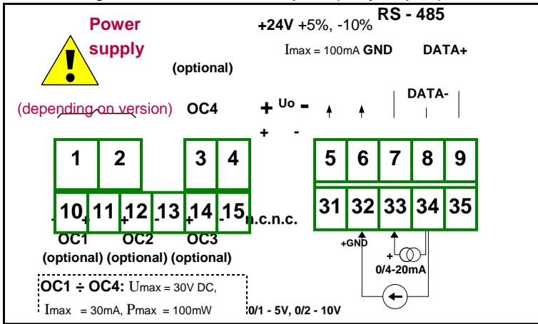
Figure 4.7. Terminals description (OC-type outputs)
