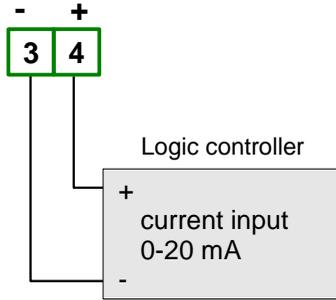
Figure 4.20. Example of active current outputs connection (for device with active current output only)
