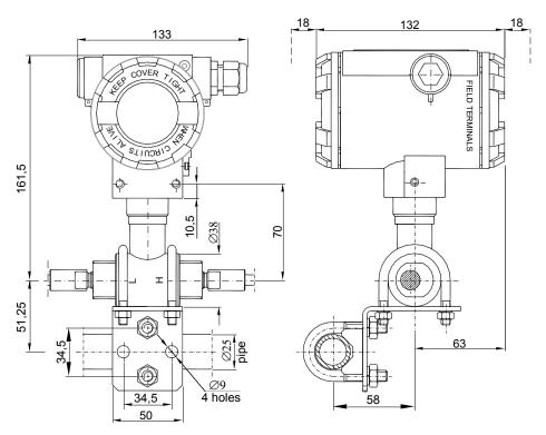
Assembly Kit ("Mounting bracket  $\varnothing$ 25" made by BASI) for fitting differential pressure transmitters with P-type connector on a  $\varnothing$ 25 pipe see catalogue cards "Fitting accessories".
