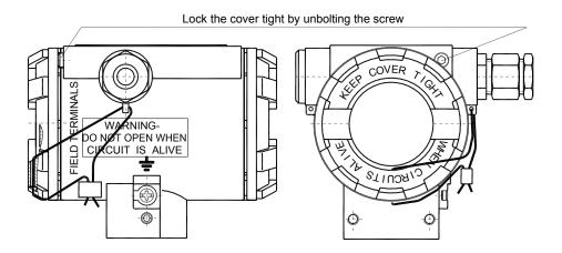
Fig. 21. How to lead the casing of BPT..., BDPT... transmitters.
