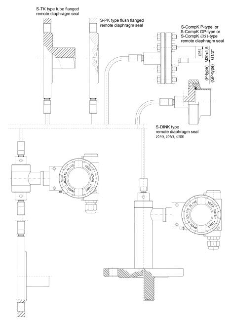
**Fig. 15**. BDPT3251-ALW differential pressure transmitter with two remote diaphragm seals (examples).
