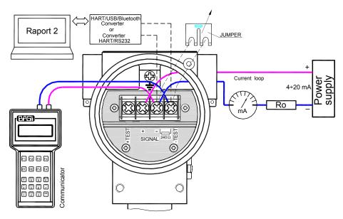
Fig.2d. The link of transmitter and communicator or converter to <SIGNAL+> <SIGNAL-> transmitter terminals in case of the resistance in current loop is smaller than 240 $\Omega$ .
