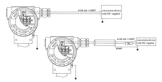
Fig. 1b. BPT3251-ALW pressure transmitter for MID application. Recommended by manufacter way of earthing to the measuring system.
