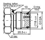
Fig.9c. CG1/2 -type connector with flush diaphragm with G1/2" thread,
