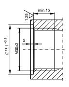
Fig.8b. Socket for CM30x2-type connector.
