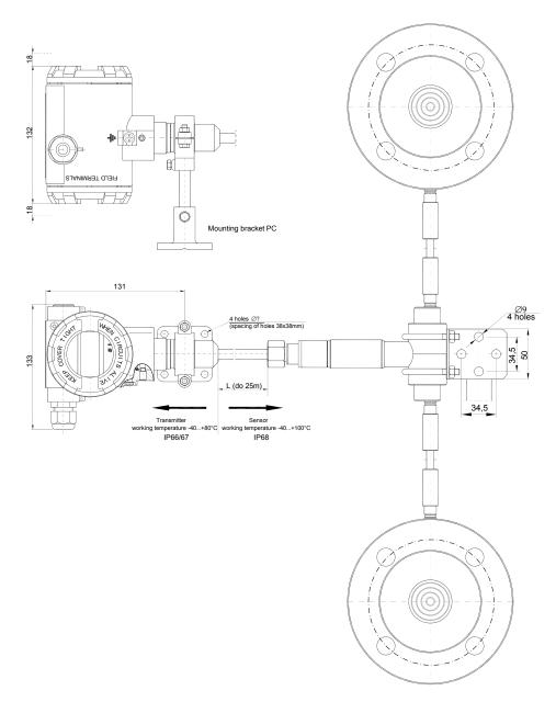
Fig. 24. An example of the differential pressure transmitter BDPT3251L-ALW.
