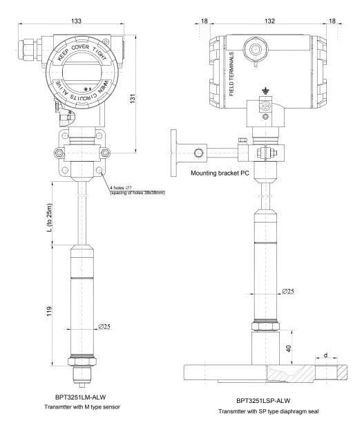
Fig. 23. BPT3251LM/LSP-ALW smart pressure or level transmitters.
