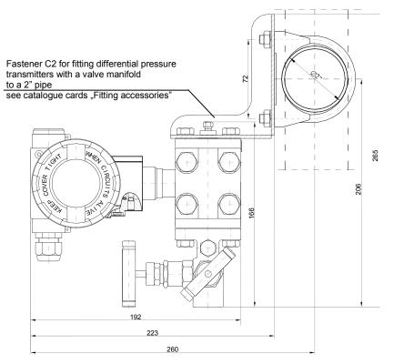
Fig. 14. Example: how to install the BDPT3251-ALW transmitter with a valve manifold to a 2" pipe.
