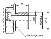
Fig.7a. P-type connector with M20x1.5 thread
