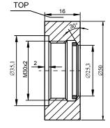
Fig.8c. Socket for CM30x2-type connector Sealing: teflon
