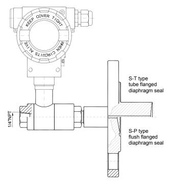
Fig. 11. BDPT3251-ALW differential pressure transmitter with a single direct diaphragm seal (example).
