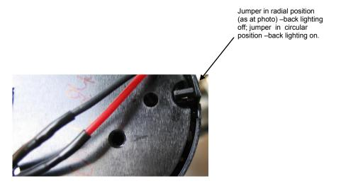
Fig. 5. Back lighting jumper view at transmitter electric board (unit display back side).
