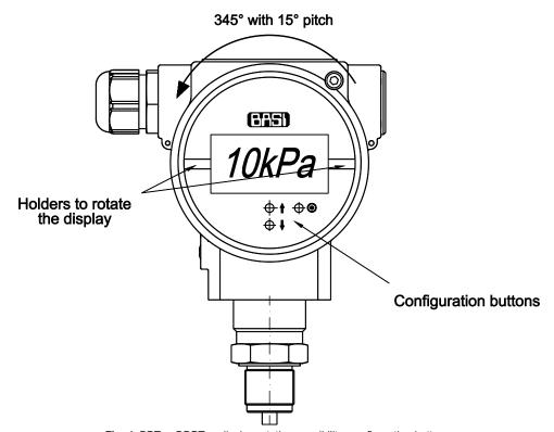
Fig. 4. BPT..., BDPT.... display rotation possibility, configuration buttons.
