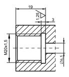
Fig.6b. Socket for M-type connector
