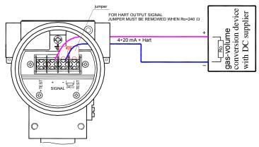
Fig. 1a. BPT3251-ALW for MID application. Connecting diagram of transmitter to powering and measuring installation.
