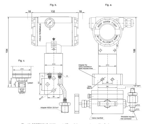
Fig. 18. BDPT3251G-ALW smart differential pressure transmitter for low ranges.
