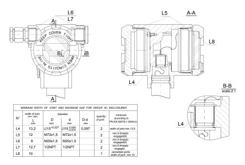
Fig. 20. The explosion - proof joints of BPT..., BDPT... transmitters.
