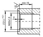
Fig.7b. Socket for P-type connector
