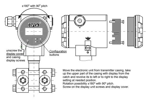
Fig. 4a. "Version SC" for BPT..., BDPT.... display rotation possibility, configuration buttons.
