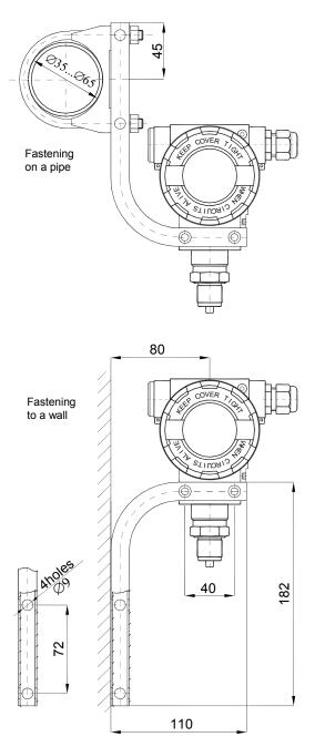
Fig. 17. Example: how to install the BPT..., BDPT... transmitter.
