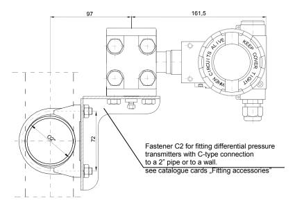
Fig. 13. Example: how to install the BDPT3251-ALW transmitter on a vertical or horizontal pipe.
