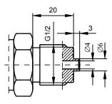
Fig.9a. G1/2 -type connector with G1/2" thread,
