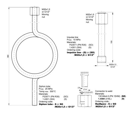
Fig. 25. Additional equipment for fitting of pressure transmitters.
