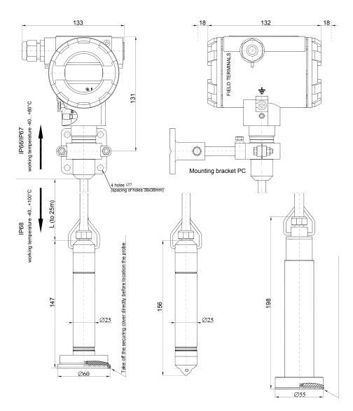
Fig. 22. BPT3251L-ALW ... smart level transmitters.
