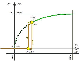
BDPT3251-ALW transmitter analog output signal with setting cutoff point in n%.
