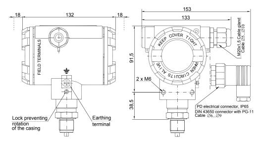
Fig. 3. BPT3251-ALW smart pressure transmitter.
