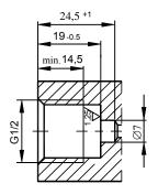
Fig.9b. Socket for G1/2-type connector.
