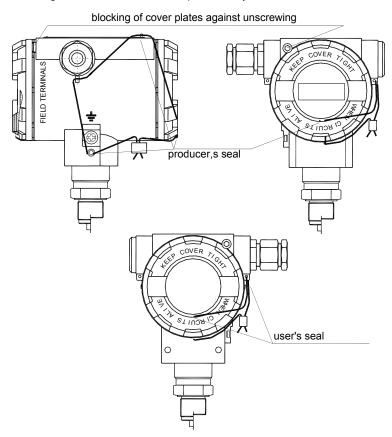
Fig 1c. BPT3251-ALW in MID application. Sealed up transmitter.
