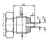
Fig.6a. M-type connector with M20x1.5 thread
