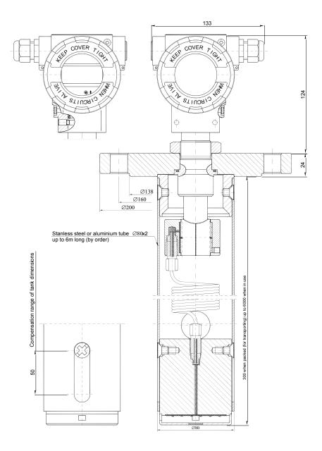
Fig. 19. BDPT3251Y-ALW smart level probe for pressure tanks.
