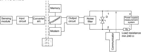
Fig. 1. BPT..., BDPT... transmitters - block diagram.
