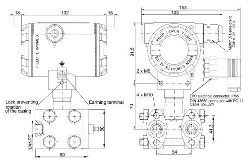
Fig. 10. BDPT3251-ALW differential pressure transmitter with C type vented covers.
