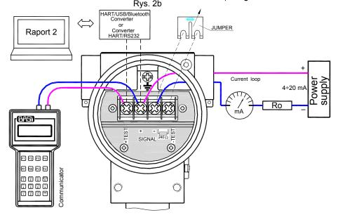
**Fig.2c.** The link of transmitter and communicator or converter to <SIGNAL+> <TEST+> transmitter terminals in case ofR resistance in current loop is smaller than 240 $\Omega$ .
