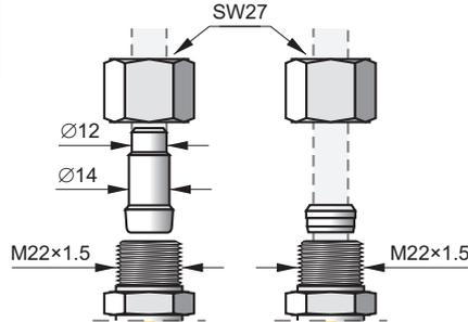
Connector for impulse line, made from 316ss stainless steel with a clamping ring:
