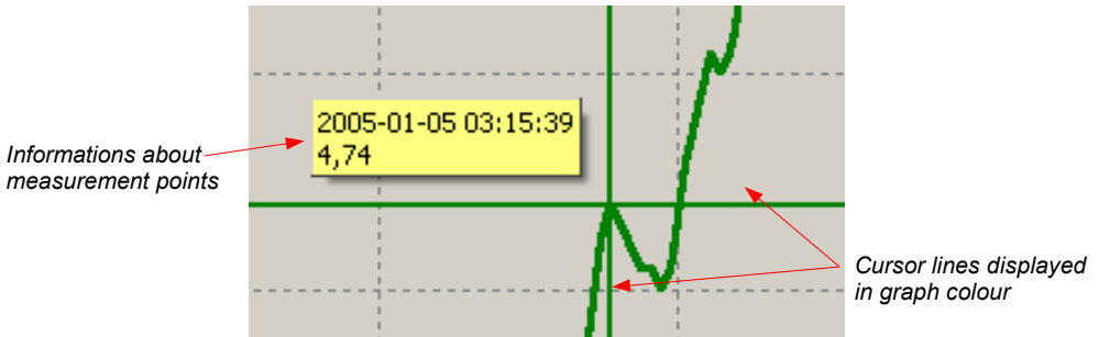
Fig. 3.9. Graph with special tracking cursor
