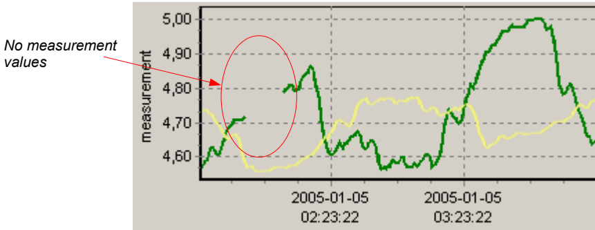
Fig. 3.10. Interruption in the graph (e.g. sensor fault)
