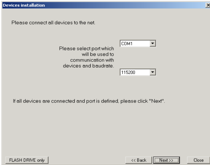
Fig. 2.1. Selection of serial port and baud rate
